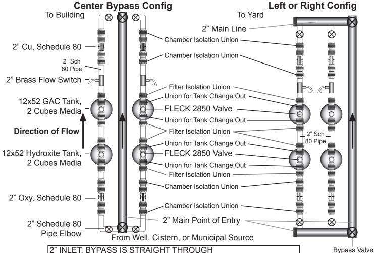
2" INLET. BYPASS IS STRAIGHT THROUGH
