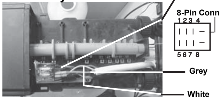
Figure 1A. Activating Your ECOsmarte® Control Valve. The ECOsmarte Control Box Connector Requires you to connect the white and grey leads from control box to pin 2 and 3, and the black and red from the water valve relay to pin 4 and 8. (Shown Fig 1A, Top view with cover off)
